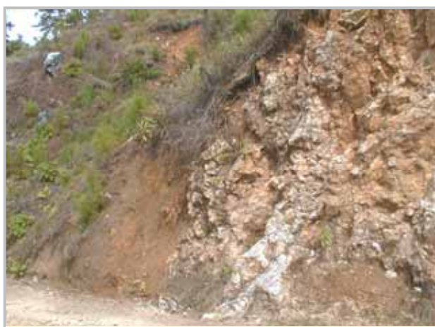
Photograph 8.4 Meteorization in lithological units promotes erosion and mass movements. Meteorization in the area occurs mostly at the local level and is not significant.
