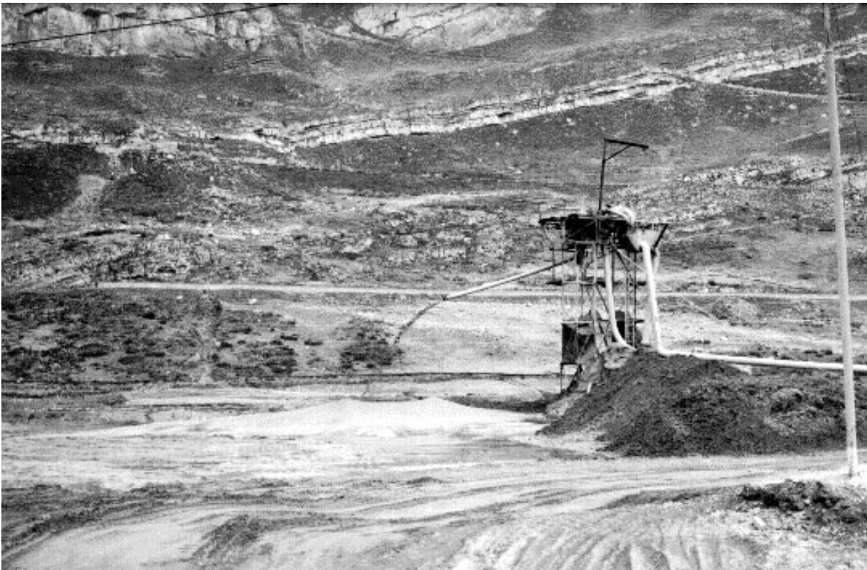
After metals are chemically extracted from ore that has been mined, the resulting wastes are called “tailings.” These tailings in the department of Junin, Peru, are a threat to nearby water sources and other pasture lands. (credit: Chris Hufstader/Oxfam America)
