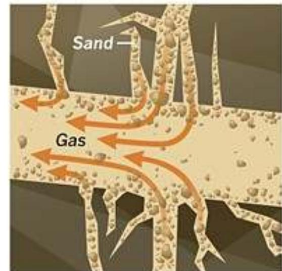
**3.** Sand flows into the fissures, keeping them open so that the oil or natural gas from the shale can flow up and out of the well.
