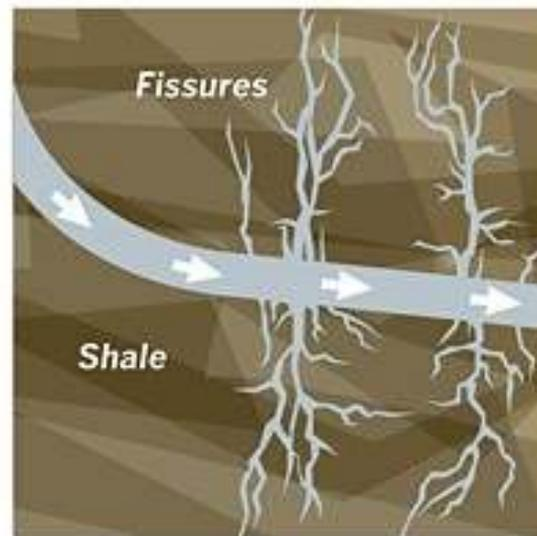
**2.** Large amounts of water, sand and chemicals are injected into the well at high pressure, causing fissures in the shale.
