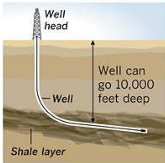
**1.** Well is bored using directional drilling, a method that allows drilling in vertical and horizontal directions to depths of over 10,000 feet.
